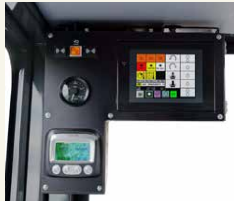
The monitoring system incorporates gauges in the cabin, allowing the operator a quick visual of engine temperature, hydraulic oil temperature and fluid levels.
