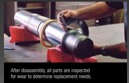
All tools are cleaned then disassembled for inspection of critical parts.
