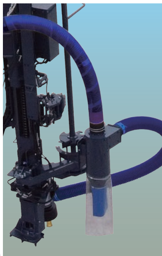
Reliable dust control system.
