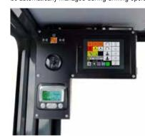
The monitoring system incorporates gauges in the cabin, allowing the operator a quick visual of engine temperature, hydraulic oil temperature and fluid levels.
